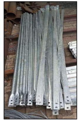
Pipe Type Earthing
